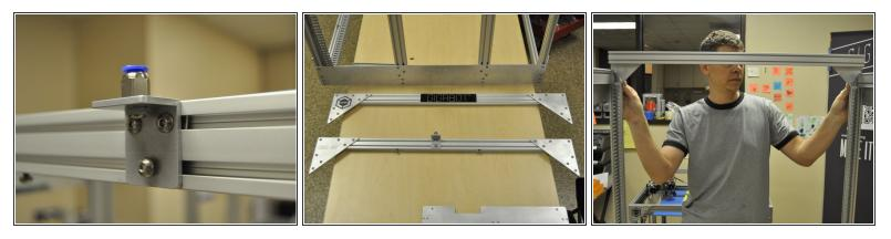
(i) Attach the re:3D Logo Corner plate to the left and blank Corner Plate to the right.
