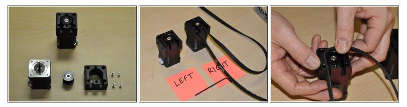
• Locate 2 Stepper motors (long ground shafts), 2 motor mounts, 2 Black GT2 timing pulleys (plastic) and 8 M3 x 8mm SHCS (socket head cap screws). See Fig. 27-1.
