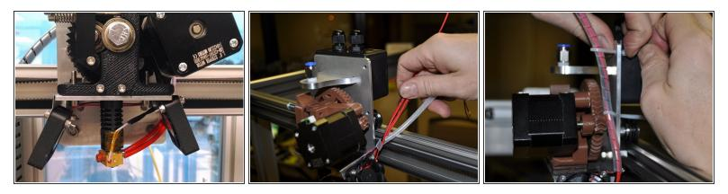
• Attach each fan by wedging in a metal plate between the cold-end and the extruder shelf. Fully tighten the BHC screws. See Fig. 36-1.
