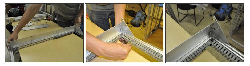
Position front/lower Cross rail assembly in front to complete the square of the frame base.
